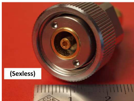
7 mm (APC-7) connector ( f_{max} \approx 18\text{-}20\text{ GHz} )
